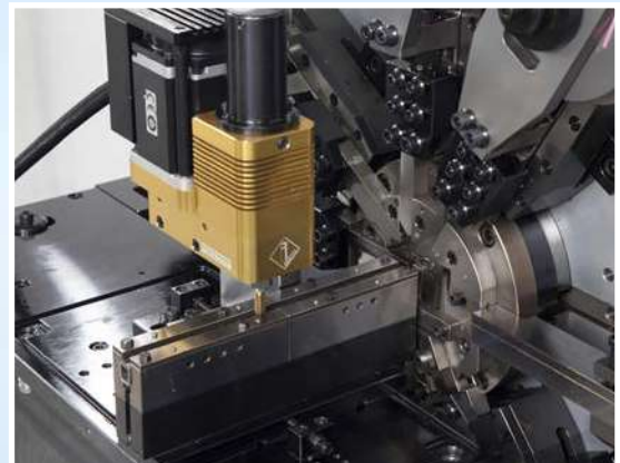
攻牙機運用 Servo Driven In-Line Tapping Attachment
